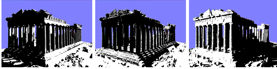
Fig. 3. Shadows precalculation: for each sun position, the scene is rendered in the Arnold Engine. In this case the engine works like a ray tracer, to determine if each single vertex is receiving light in that time of the day.
