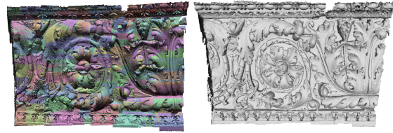
Figure 9: The coarse alignment of a portion of the archway of S. Ranieri's door, Pisa Cathedral (left). The final model after ICP and global alignment (right).
