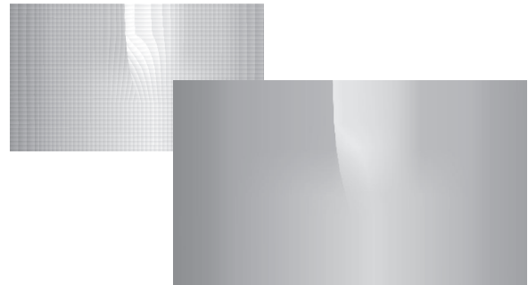
Figure 11: Here, the signal texture is a normal-map encoding a curved surface with a crease. The pinch strength is modulated from zero to one over the space of three fexels in order to make a crease start smoothly. Left: fexels are shown with a superimposed 8x8 grid, right: final result (actual screenshot).
