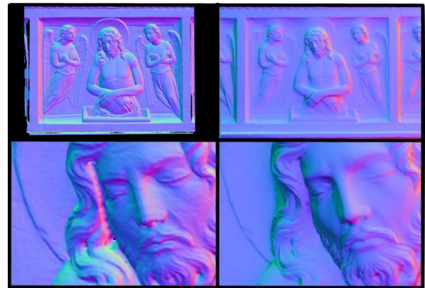
Fig. 5. Comparison between the normal maps of the 3D scanning and the PTM: full model and particular.
