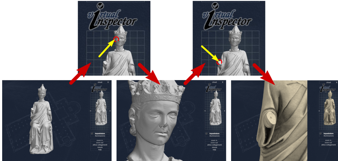
Figure 2: The new gaze point, selected by the user by a simple mouse click on the corresponding location on the dummy, is marked for illustration purposes by a red circle (see the two zoomed image fragments).
