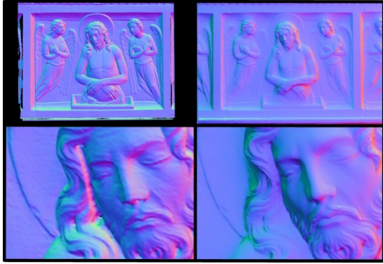
Figure 4: Comparison between the normal maps of the 3D scanning and the PTM: full model and particular.
