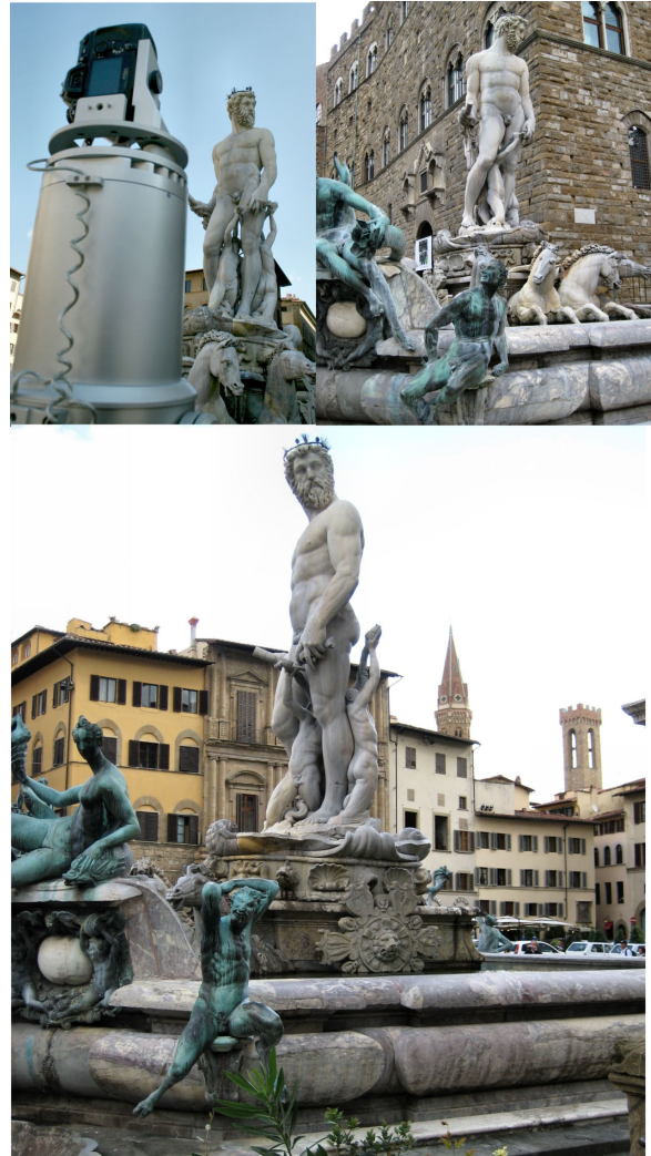
Figure 1: Three views of the Neptune fountain. In the Top Left: the Time-Of-Flight scanning device during the acquisition
