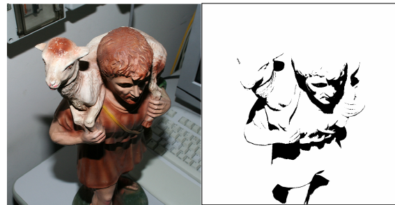
Figure 4: An example of shadows detection: left, the original image; right, the shadow detection map.
