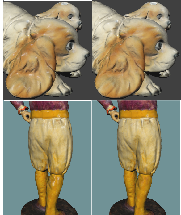
Figure 6: Details of two colored models, visualized with no illumination (only color values assigned to vertices): on left, the result without highlights removal, on right the model after applying highlights removal.
