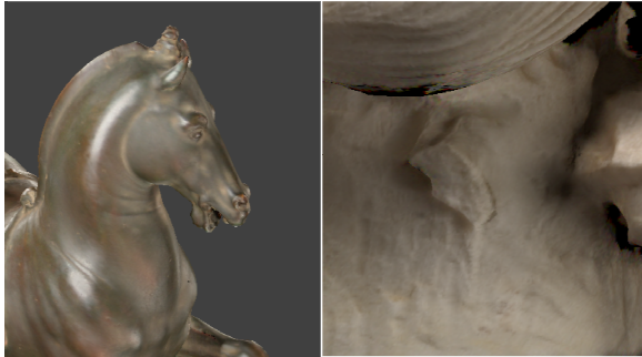
Figure 5: Details of two colored models produced with [CCCS08] (no flash images), visualized without illumination and shading (only color values assigned to vertices): multiple highlights show up on the digital models (left); the presence of shadows and different illumination between photos generates a non completely continuous color (right).
