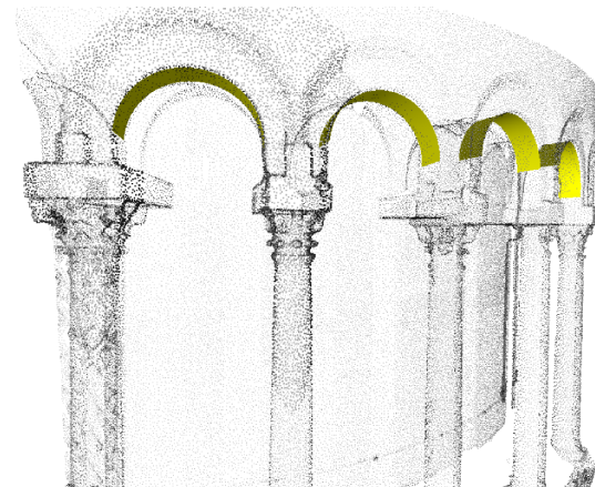
Figure 7: Above: example of selection of stair steps: (a) mouse gesture for the first step (b) fitting (c) mouse gesture for replicating the fitting (d) result. Below: final results for a set of arcs.
