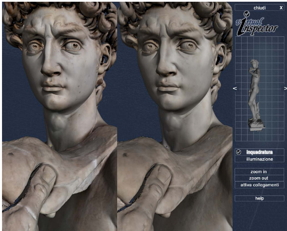
Figure 1.9: The David model is shown with color mapping; on the left is the pre-restoration status (61 images mapped), while the post-restoration status is shown on the right (another set of 68 images). The two colored David models are rendered in real time with the Virtual Inspector system [56].
