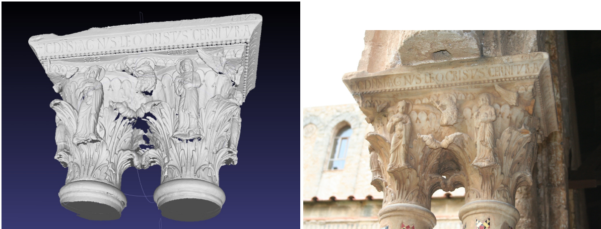
Fig. 1 A rendering of an incomplete model, where part of the geometry could not be acquired with laser scanner (missing regions are easily detectable as blue holes) and a photograph of the real artifact.
