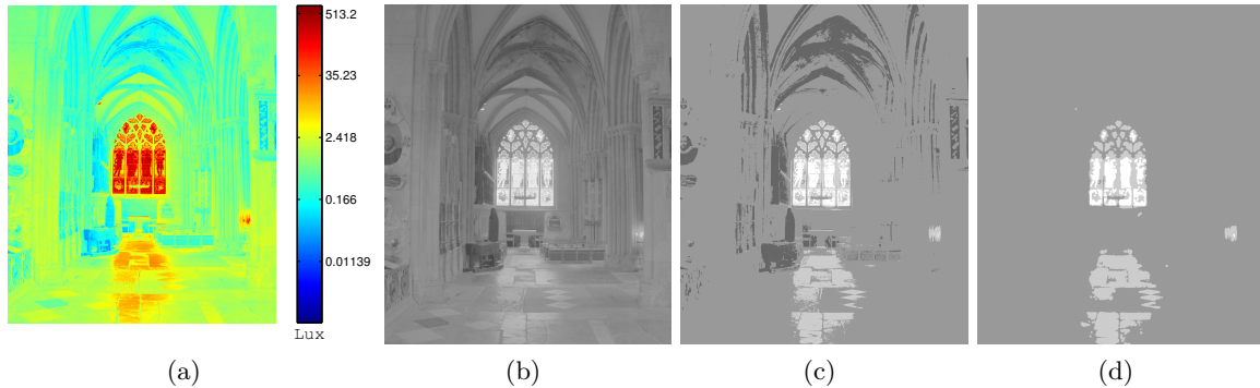
Figure 2. An example of CDM computation: (a) The input HDR image, tone mapped using Reinhard et al.’s operator 20 for visualization purposes. (b) The L_{log} of (a). (c) The rounding on (b). (d) The final CDM after merging segments with a mean distance less than 1. The number of segments in this example is 3.
