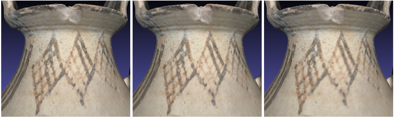
Fig. 3. Left: Brute force method. Center: Hierarchical template matching. Right: Floating Texture's optical flow implementation [31]. Note how even though the third method better preserves the borders (top of the vase), the patterns in the center of the figure are sharper with the first two methods.
