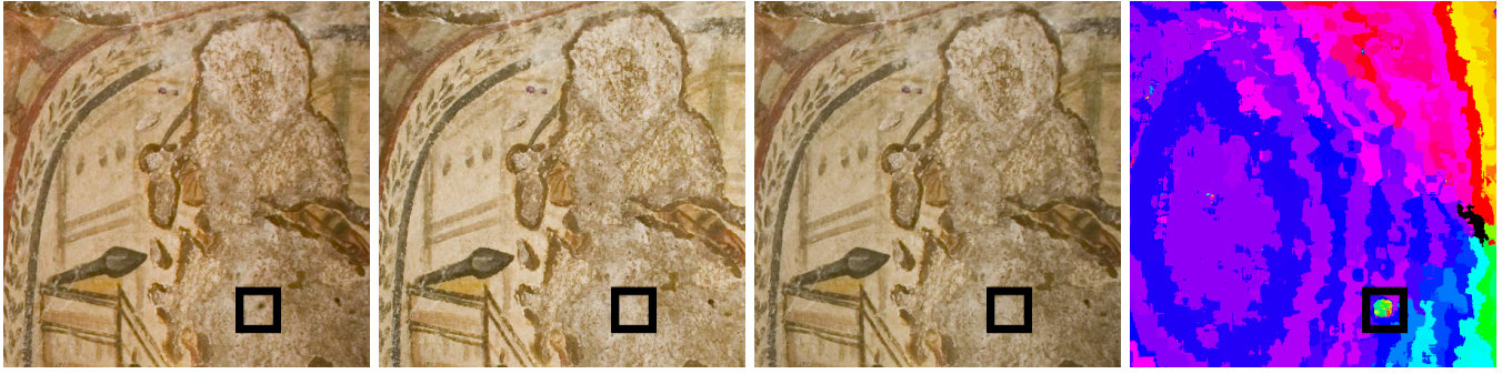
Fig. 5. Sequence of detail images from the flow calculation of the Painted Catacomb. From left to right: original image (target), projected image (source), target image warped with flow, and the flow field. Note that the flow is also able to remove noise (inside the black square in evidence) from the original image. The flow pattern indicates that there is not only a translation between the images, but also a radial distortion possibly caused by the camera lenses or image projections.
