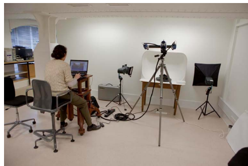
Figure 1: 3D scanning setup in the photographic studio of the V&A museum
