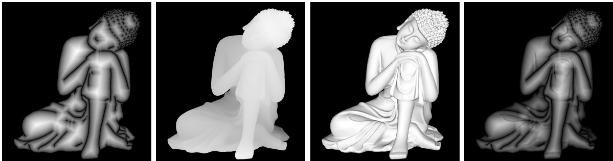
Figure 2: Quality computation: (Left) map of the border distance from the depth discontinuities; (Left-Center) depth map; (Right-Center) dot product between the normal and the view direction; (Right) final quality.
