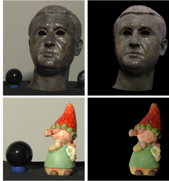
Figure 4: Comparison between an image of the object acquired in a different lighting environments (Left) and the rendering with our SVBRDF approximation (Right): (Top) HEAD; (Bottom) DWARF.
