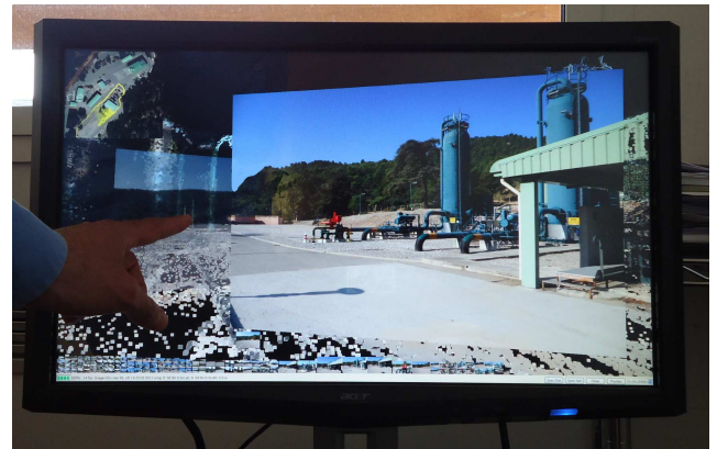
Figure 6: Highlight of the next image candidate Live navigation in the Geomethane scenario. Touching a point in bottom left corner of the screen the most representative image for that spatial place is highlighted. With a double click the camera automatically moves to the point of view from which the candidate image has been taken.
