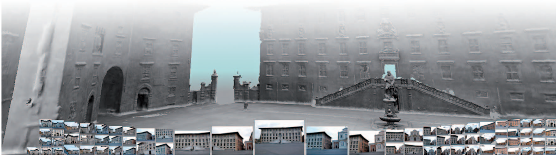
Figure 6. The thumbnail bar. This focus-and-context image browser arranges image thumbnails into stacked piles. The focus image is the largest thumbnail, in the middle of the bar. The others get clustered into piles whose size decreases and whose depth increases as the piles get farther from the focus. Images in the same pile are semantically close. The interface includes mechanisms to scroll, select, and preview images.
