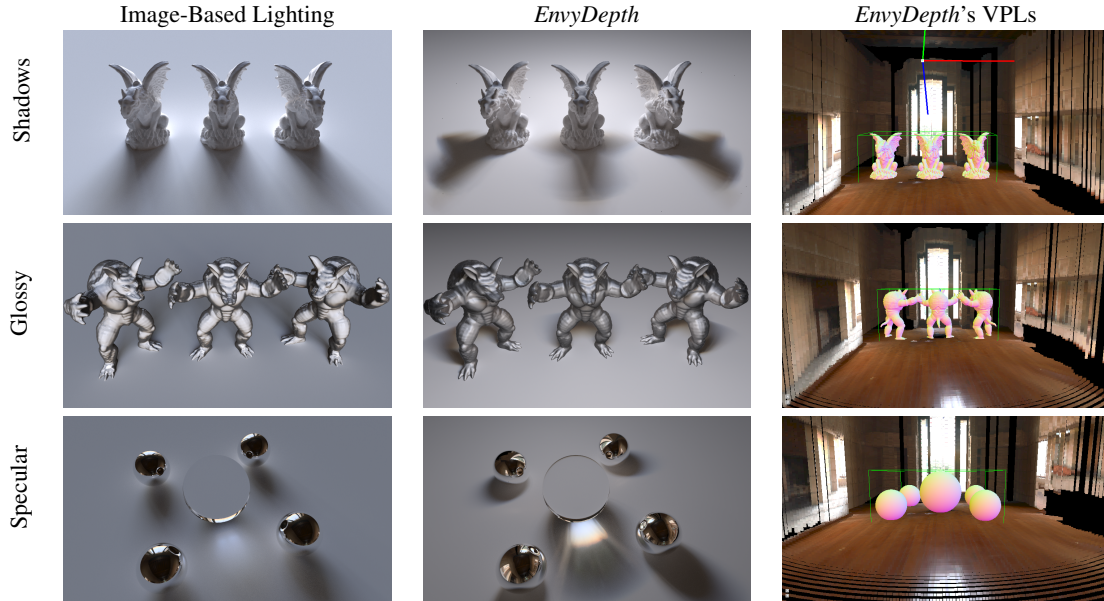
Figure 5: A comparison of our method with image-based lighting [Deb98] using the Ennis environment map. In this comparison, we tested for different spatial effects such as: local shadows (Shadows), glossy BRDF (Glossy), and full specular effects (Specular).
