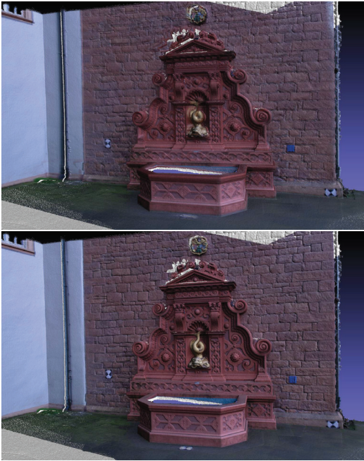
Fig. 14 (Top) Color projection for Fountain dataset, using ground truth camera data. (Bottom) Color projection using the camera data estimated with the proposed method.
