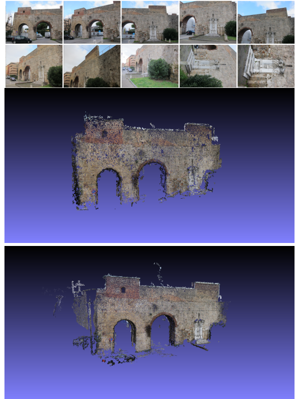
Figure 8. The City Wall test set. First row, an example of some of the images used for the reconstruction. Second row, the reconstruction obtained with Our method (28 images). Third row, the reconstruction obtained with VisualSfm+PMVS2 (32 images) [22]
