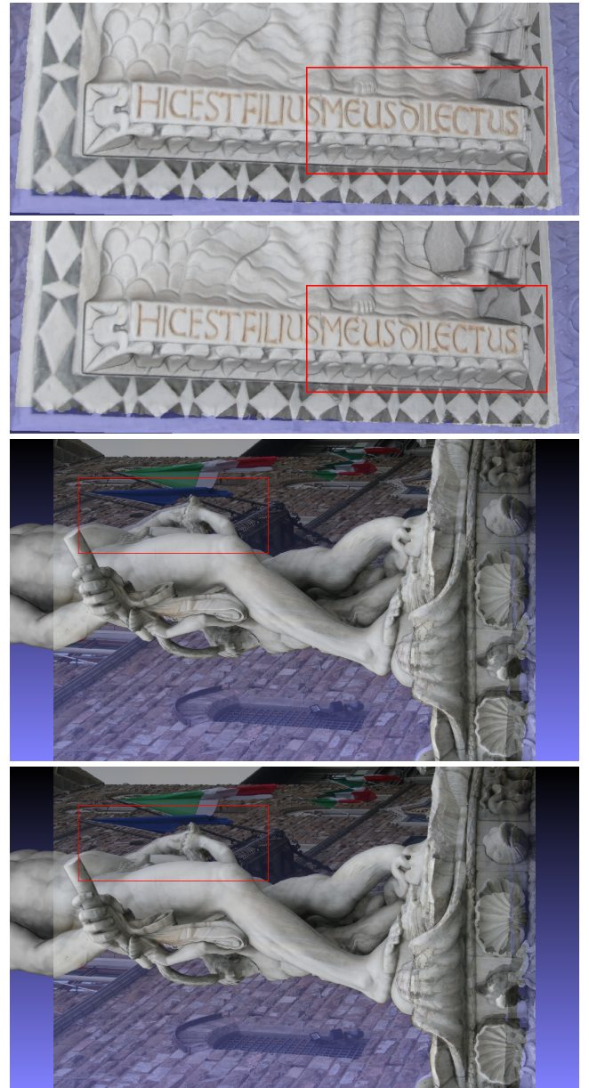
Fig. 3. Two examples of the refinement of single images after the application of our method, showing an image with the 3D model in transparency. In the first one (first and second row) small details are better aligned. In the second one (third and fourth row) the silhouette is better matched.
