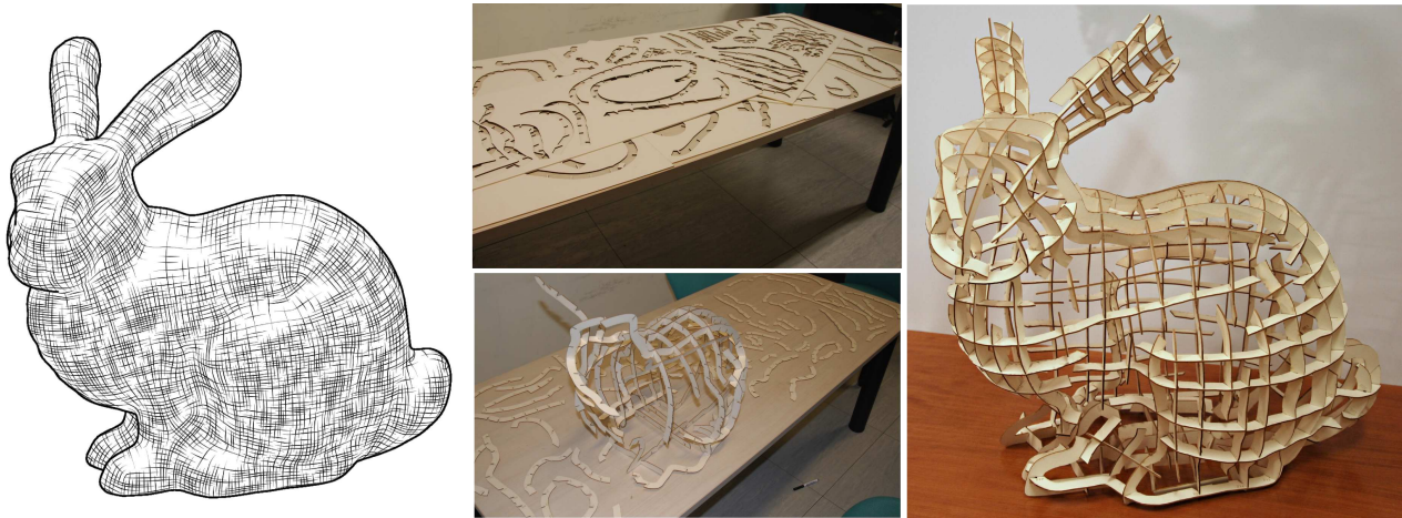
Fig. 1. Given a 3D shape with a smooth cross-field, we generate a set of planar slices that can be interlocked in a self supporting structure.
