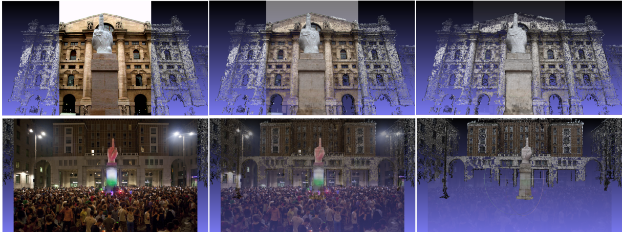
Figure 9: Two images taken from community collections, aligned with the reference point cloud.
