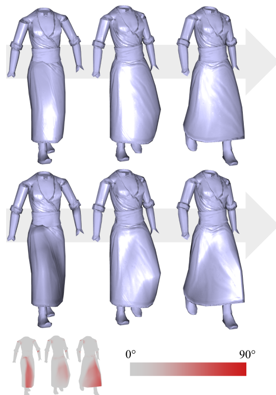
Figure 1: Lighting a skinned low-poly, normal-mapped model. Top sequence: the standard method produces inaccurate normals that makes the skirt look flat. Mid sequence: our algorithm produces an accurate lighting which better conveys the shape of the skirt. Bottom: differences in normals. See also attached video.
