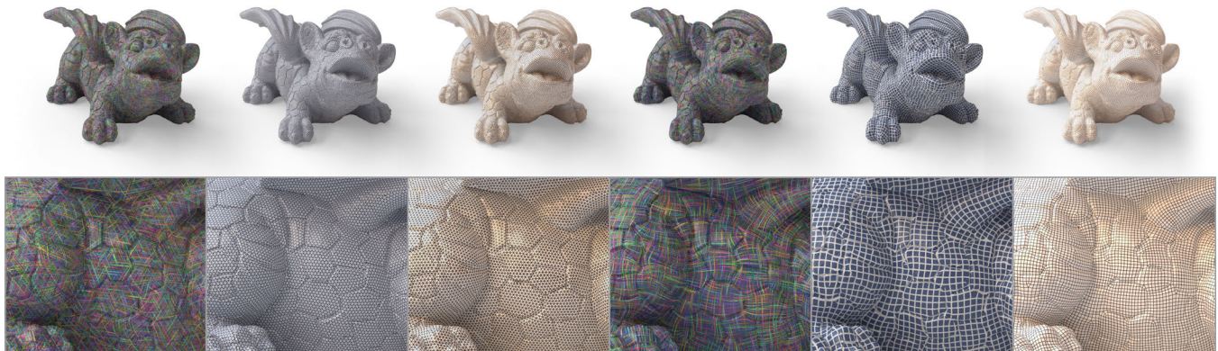
Figure 1: Remeshing a scanned dragon with 13 million vertices into feature-aligned isotropic triangle and quad meshes with \sim 80k vertices. From left to right, for both cases: visualizations of the orientation field, position field, and the output mesh (computed in 71.1 and 67.2 seconds, respectively). For the quad case, we optimize for a quad-dominant mesh at quarter resolution and subdivide once to obtain a pure quad mesh.
