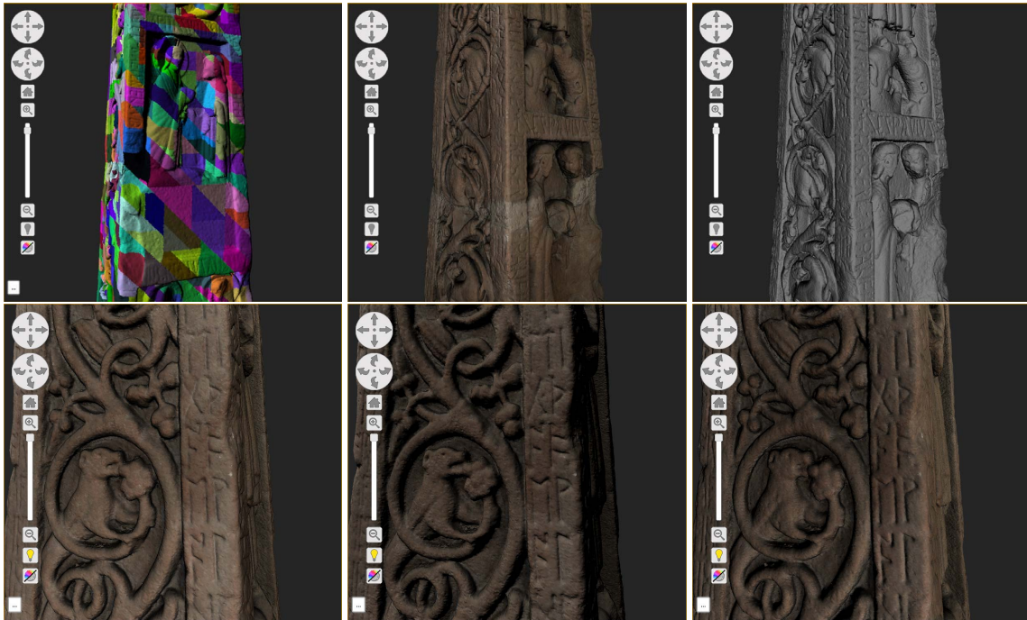
Fig. 3. Images grabbed from the web-based multiresolution 3D model of the Cross. Top left: the patches used by the multiresolution rendering engine in this specific frame. Top middle: the geometry rendered with photographic color. Top right: the same geometry rendered using a simple Lambertian shading (no color). Bottom row: changing the light direction, to simulate raking light, helps to improve insight of the small carvings, especially the carved runes.
