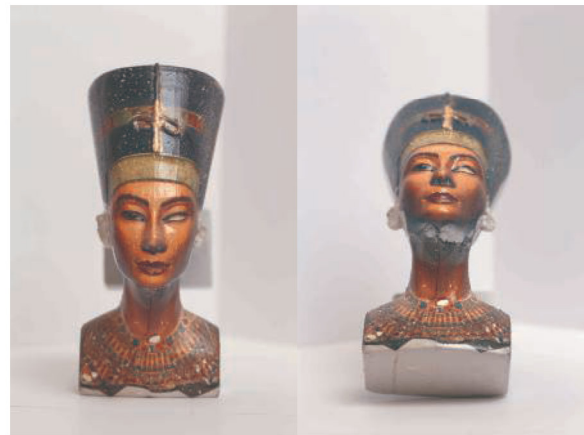
Figure 10: A photograph of the textured Nefertiti model. The film stretches and deforms for dipping angles with the surface that are lower than 45 degrees (left), but tears uncontrollably for higher angles (right).
