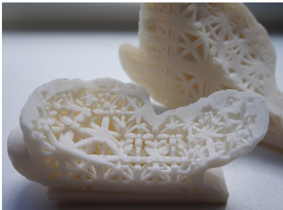
Figure 2: The Stanford bunny printed in ABS using an open cellular structure infill.
