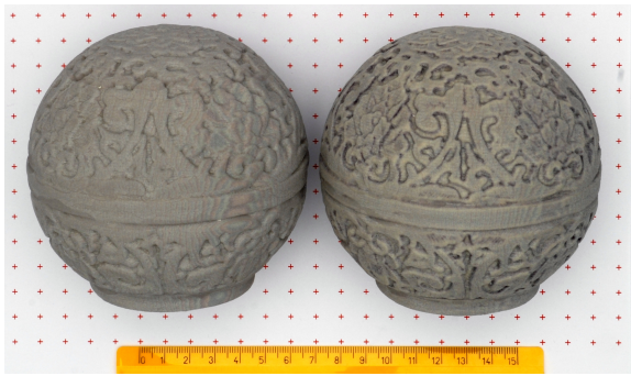
Figure 4: By controlling the diffuse colour during the fabrication process the subsurface scattering effect that reduces the perception of small scale geometry can be counterbalanced.
