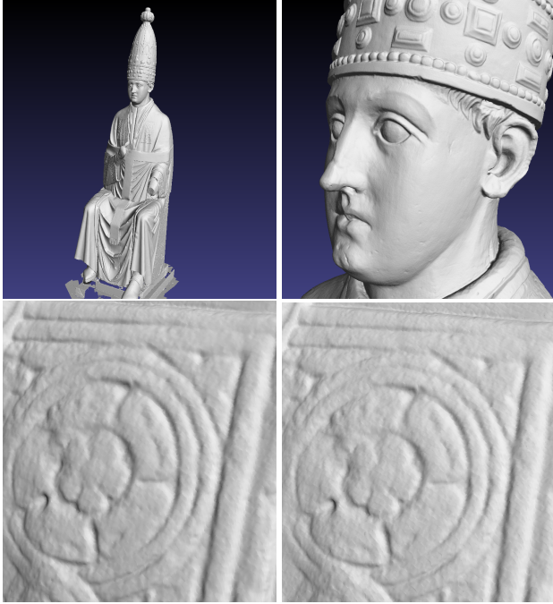
Figure 7: Bonifacio rendered in a browser: original PLY file, 84M triangles, 1.6GB; uncompressed model, 2.54 Gb; compressed model, 158 Mb. Top left: the full compressed model, top right: a detail. Bottom left: a detail of the uncompressed model. Bottom right: the same detail of the compressed model
