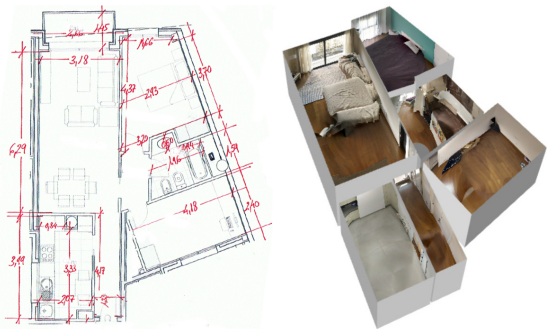
Figure 6: Apartment with 7 rooms (Tab. 1 House2). On the left the blueprint assumed as ground-truth with its real measures indicated by the designer. On the right our reconstruction.
