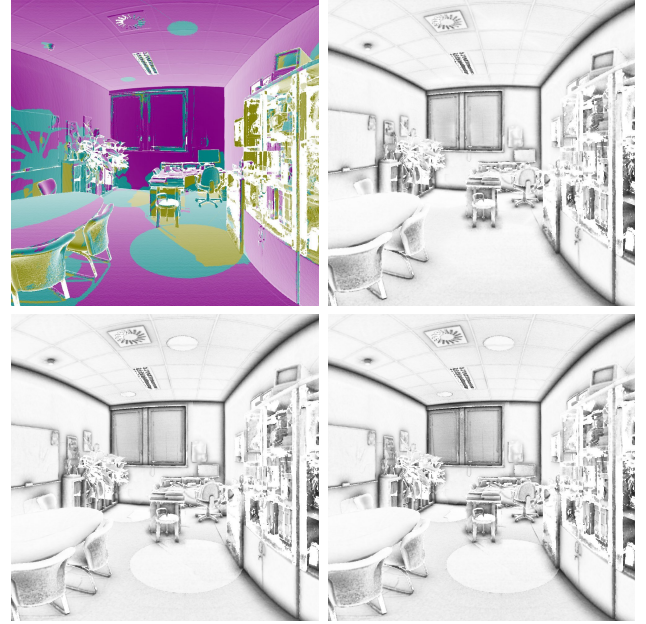
Figure 5: Effect of the border weight w_b on the computation of the MVAO: (Top-left) image with the color encoding of the scan coverage for each point (yellow = one scan, light blue = two scans, pink = three scans); (Top-right) MVAO using our weighting function in Equation 9; (Bottom-left) MVAO using the weighting function proposed in [VPG13]; (Bottom-right) MVAO using our weighting function without the border weight w_b .
