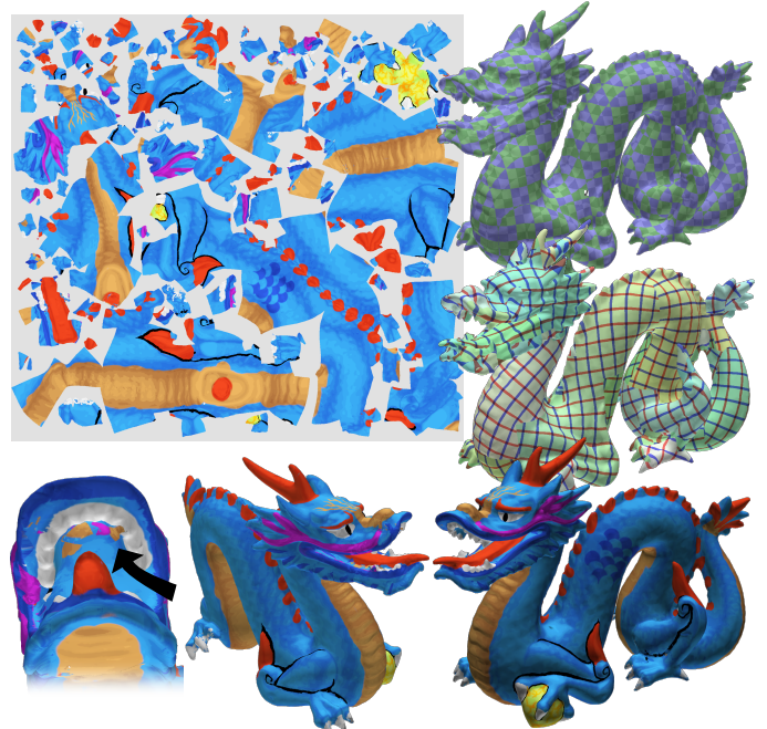
Figure 17: A failure case. This “dragon” model is not a good candidate for our UV-map representation: the thin parts, e.g. in the mouth, cannot be parametrized without loss of injectivity. The resulting UV-map has four cases of partially self-overlapping charts, producing local artifacts when the artist-painted texture is mapped on the mesh (e.g. see inset, lower right—and the attached demo).
