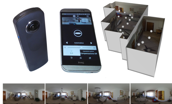
Figure 1: Modern mobile panoramic cameras driven by smartphones (top left) can easily capture sequences of spherical images (bottom), which can be exploited to automatically reconstruct structured 3D models (top right).
