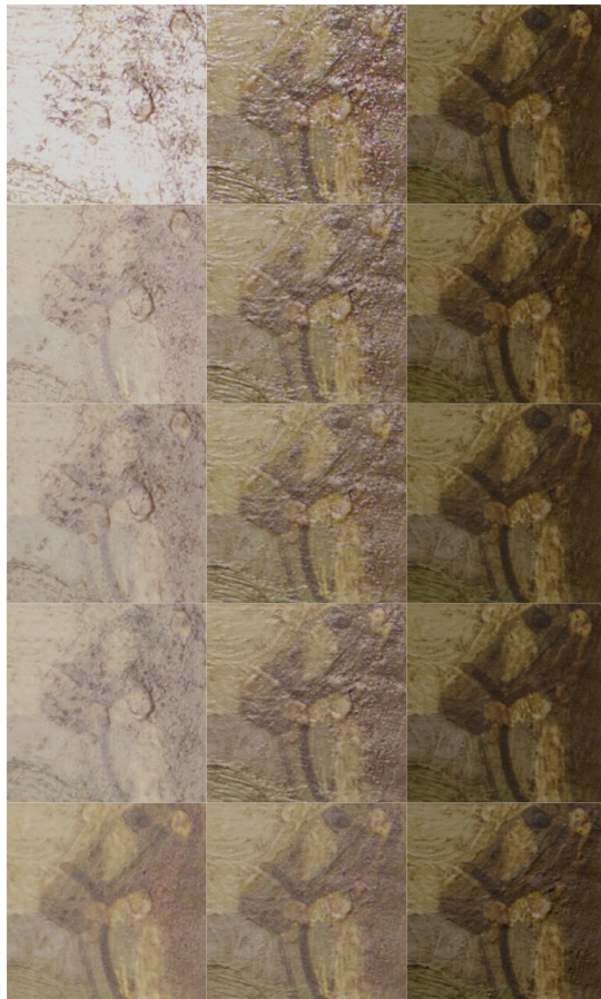
Figure 5: Rows from top to bottom: original images, BILIN-EAR27, RBF27, YCC711, HSH. The original images shown are the number 0 (column 1), 17 (column 2) and 18 (column 3) of the dataset. Note that the image number 0 has a very strong specular highlight. YCC711 is able to catch this behavior better than the HSH, even if its size is about 50% of the HSH.
