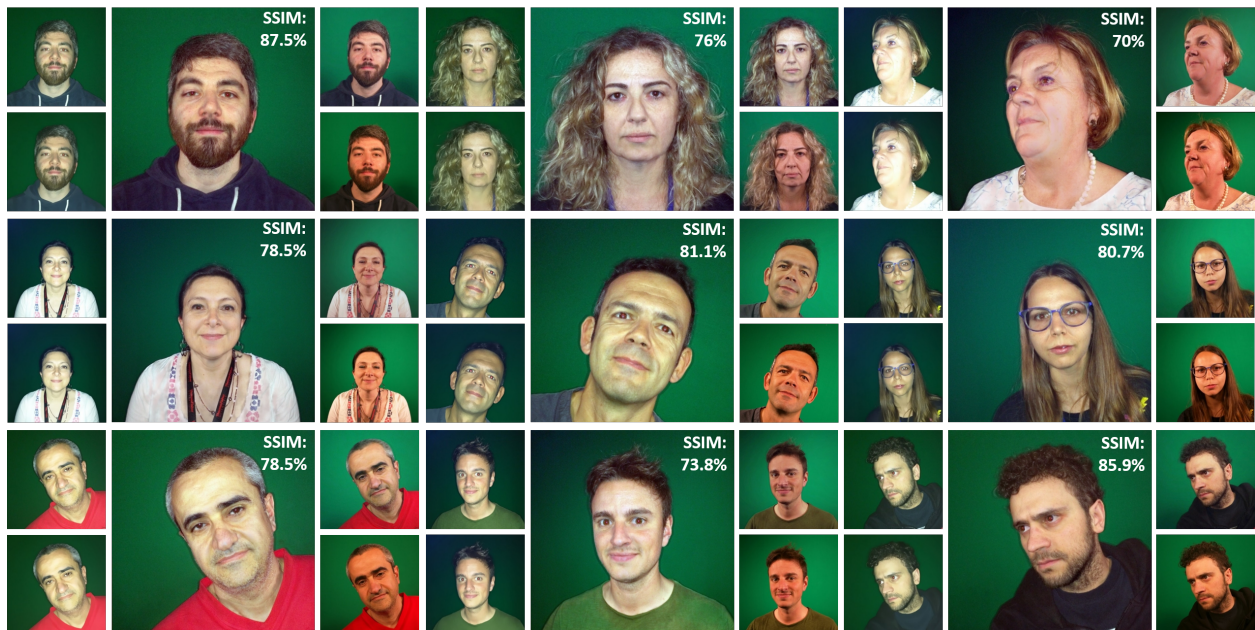
Figure 5: Samples of validation data. Each group of images is composed of: the original image taken with the smartphone flash (top left); the flash image to which the bilateral filter was applied (bottom left); the image reconstructed by the difference prediction of the CNN (center); the ground truth reconstructed (top right); the ground truth (bottom right). The SSIM was computed by comparing the central image of each group and the image at top right.
