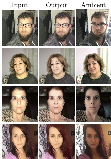
Figure 3: Results of our approach on real selfie images of the dataset provided by Y.Aksoy et al. [7]. The first column represents the input of our neural network, the column center represents our result and the last column represents the no flash ambient image.
