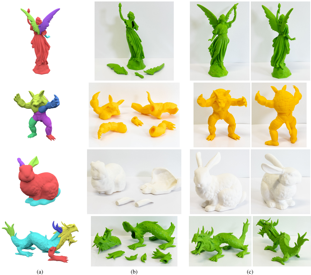
Figure 11: Some successful examples of segmented, fabricated and assembled objects: (a) segmentations; (b) 3D printed and oriented shell pieces; (c) the assembled model. It can be seen how cuts tend to hide into the object features.
