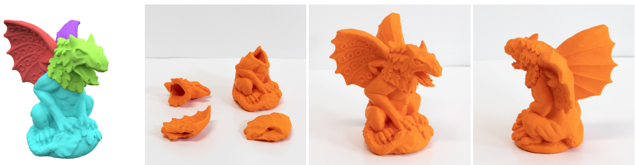
Figure 1: Our method partitions an input object into a small number of simpler parts, which can be 3D printed with few supports, and such that the gaps separating parts have a low visual impact on the assembled object.
