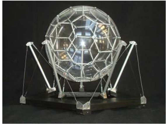
Fig. 1 1:10 Scale model demonstrator of the SGS (model by the author Froli)
