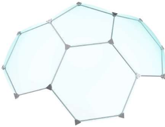
Fig. 2 Concept of structural system: bent panels and wire frame steel mesh are connected at the nodes; the panels' edges are then sealed for waterproofing
