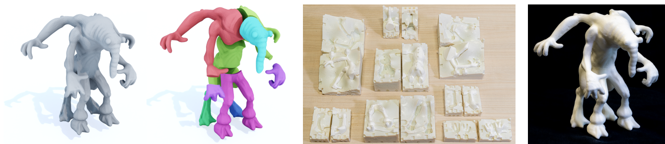
Fig. 1. Given a closed 2-manifold mesh, we split it automatically into double height field (DHF) components that can be fabricated using two-piece rigid casting and assembled afterwards.
