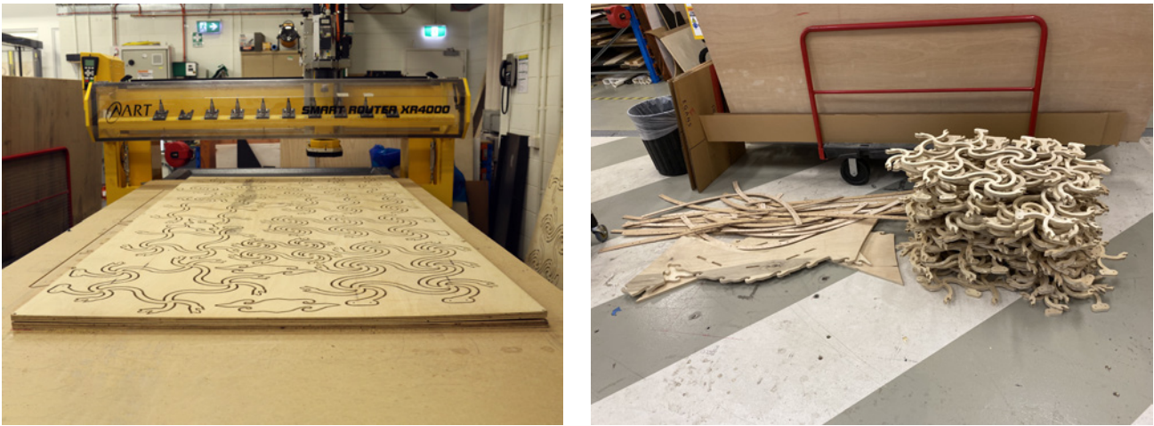
Figure 18: Fabrication of the demonstrator: CNC cutting and components after sanding.
