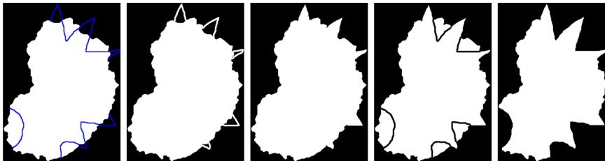
FIGURE 4 The algorithm of the Edit Border tool explained. From left to right: (1) The binary mask and the input edit curves (drawn in blue) snapped to the mask. (2) Edit curves are first drawn in white. (3) Filling of the subtended regions. (4) Edit curves are redrawn in black. (5) The largest connected component becomes the final mask. Note that the black and white lines are thin to enable pixel-level precision during the mask processing. We thicken the lines to improve the clarity of the figure [Color figure can be viewed at wileyonlinelibrary.com ]
