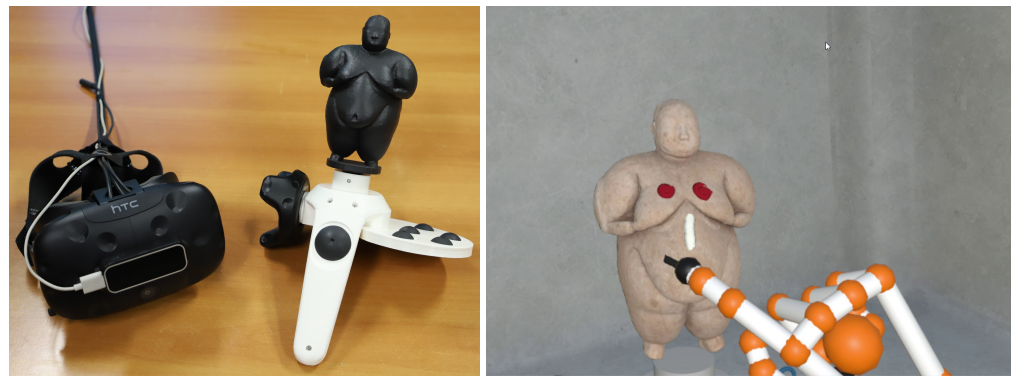
Figure 1. (Left) Photos of the hardware of the system: HTC Vive, LeapMotion, Vive Tracker, the 3D-printed support with the replica that hosts the controller for capacitive touch sensing. (Right) Example of a painting session.
