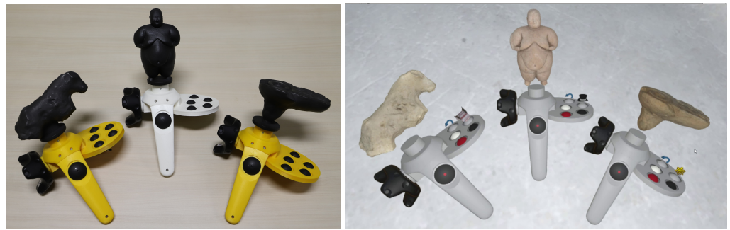
Figure 11. Photo of the devices made for the three test objects and rendering of their VR counterparts.
