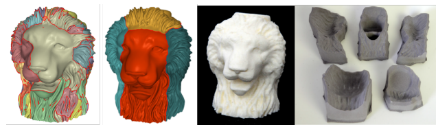
Figure 10: An example demonstrating the multi-piece molds generation algorithm from Herholz et al. [HMA15]. From left to right: the output of the method when no undercut constraint violations are allowed, the regularized output with surface deformation, the resin cast, and the mold pieces.
