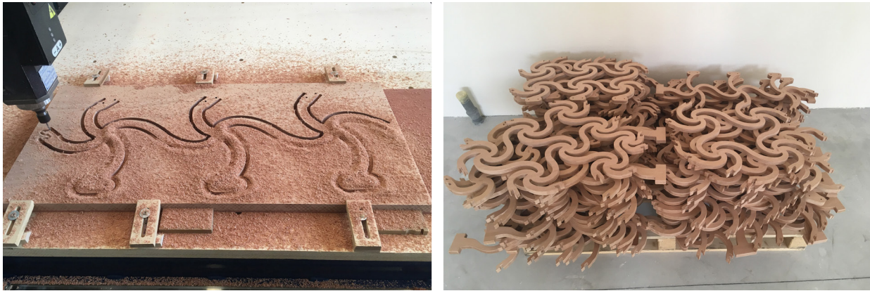
Figure 14: Fabrication of the FlexMaps patches
