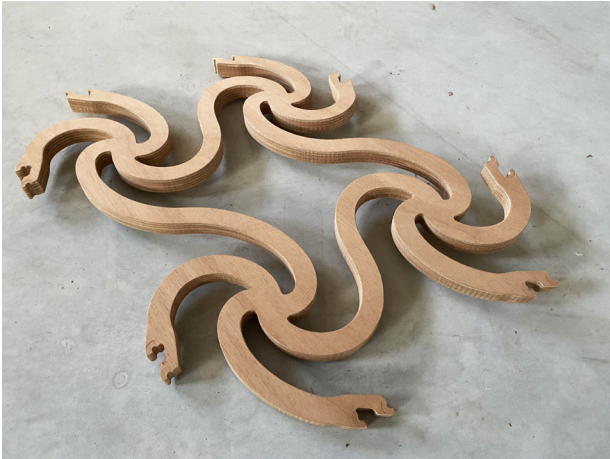
Figure 18: Inelastic deformation of patches after the Biennale exhibition
