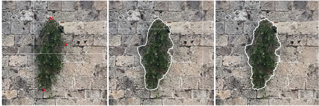
Fig. 3. The 4-clicks segmentation tool in action. (Left) The user marks the extreme points of the area to be segmented helped by the cross-cursor. (Middle) The Deep Extreme Cut CNN automatically traces the boundaries. (Right) The Refinement tool can then be used to obtain a more precise segmentation.
